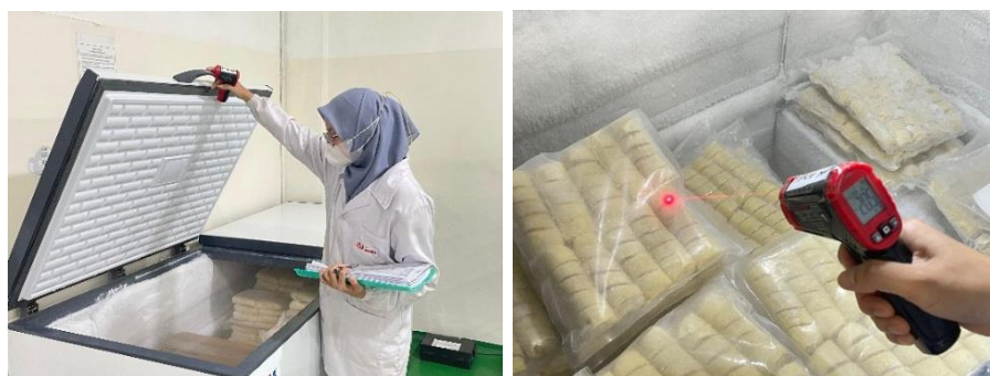
Gambar 3. Monitoring Suhu Freezer Penyimpanan
